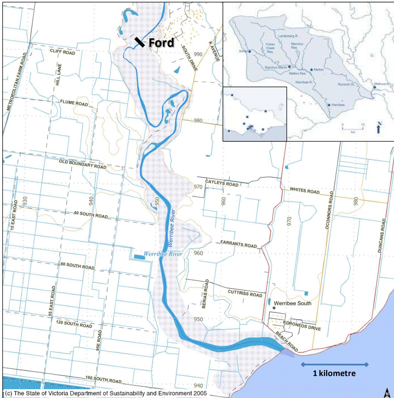
Figure 1-2. Location of the Werribee River estuary, from downstream of the ford. Shading indicates the 1 in 100 year floodplain.
