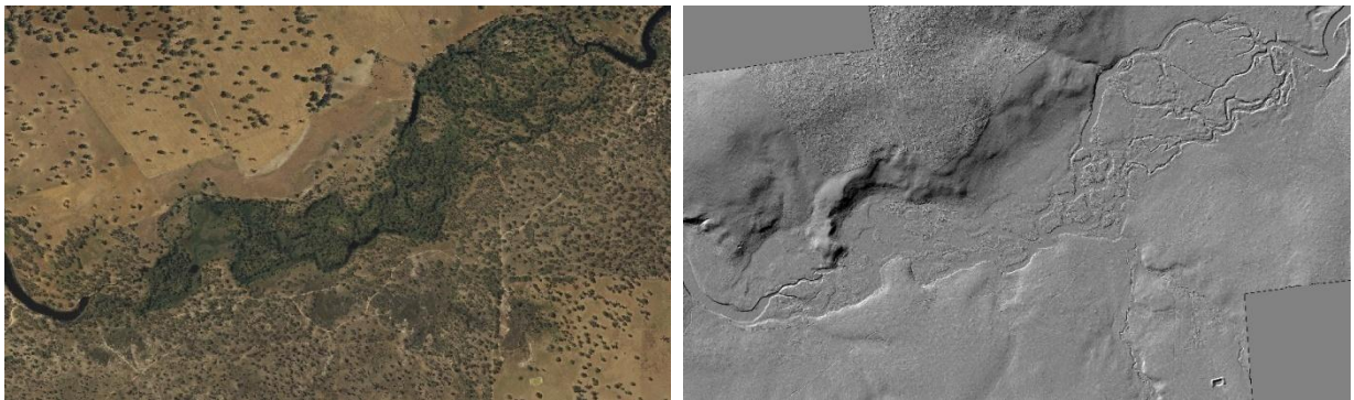
Figure 22. Upstream of Fulhams Bridge (flow right to left), Note the transition between a well-defined single thread channel, to multiple channels then a floodout feature with no defined channel before forming a single thread channel again
