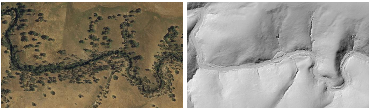
Figure 23. Section of reach 1b which has incised into the bedrock plains leading to valley confinement (flow direction right to left). Note the depositional features at the valley margins.
