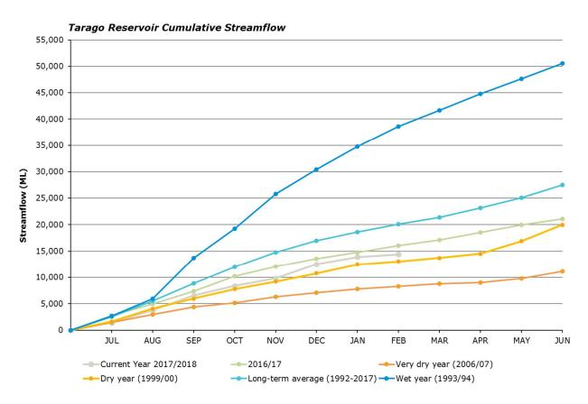
Figure 1.7: Cumulative streamflow at Tarago Reservoir under different scenarios (dry to wet years)
