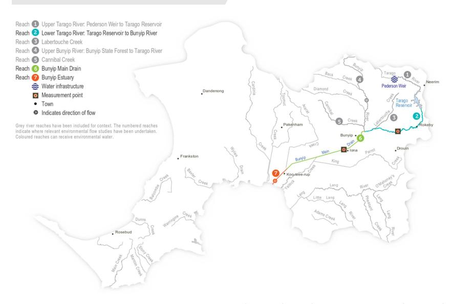
Figure 1.1 : Tarago and Bunyip reaches for environmental water management. Reach 2 (Lower Tarago), Reach 6 (Lower Bunyip - Bunyip Main Drain) and Reach 7 (Bunyip Estuary) can receive environmental water. Source: VEWH (2016).
