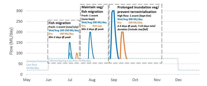
Figure 1.3 : Schematic illustrating Reach 2 flow recommendations for Winter/Spring Fresh and High Flows in wet/average and dry years.
