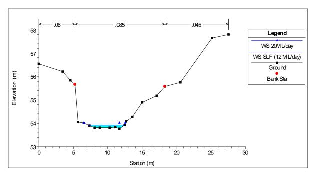
Figure D.1: Plot showing increase in width of wetted bed/riffle and flow depth that would result with an increased in volume of recommended low flow from 12 ML/Day to 20 ML/day at Reach 2 Flows Assessment Site. Width of wetted bed/riffle increased from 5 m to 6 m and depth of flow increased from 10-15 cm to 15-20 cm.
