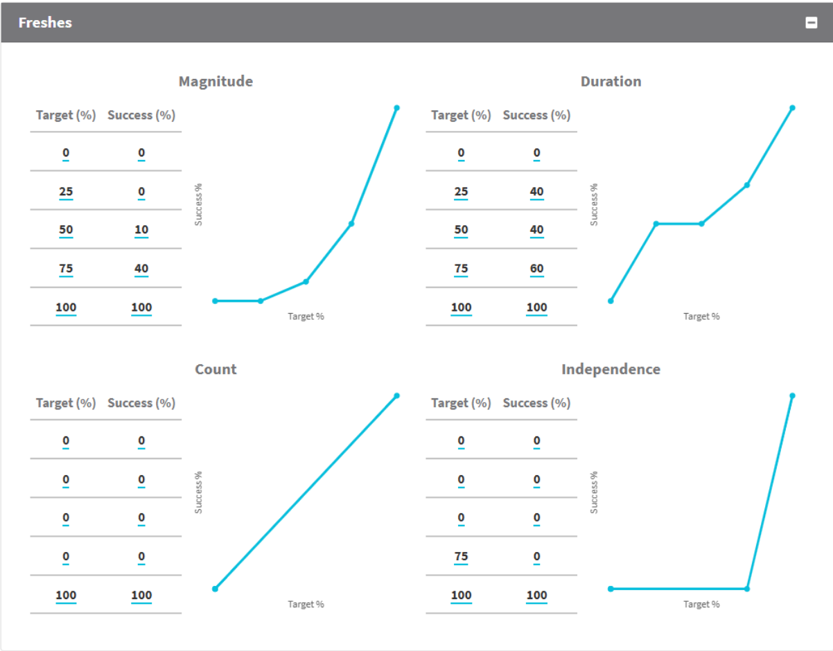
Figure 28: A screenshot from eFlow Projector showing how modelled flow as compared to the target flow (i.e. flow target) is converted to a measure of success for freshes
